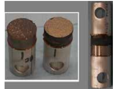
Typical ASTM C633 Adhesion Strength Test
